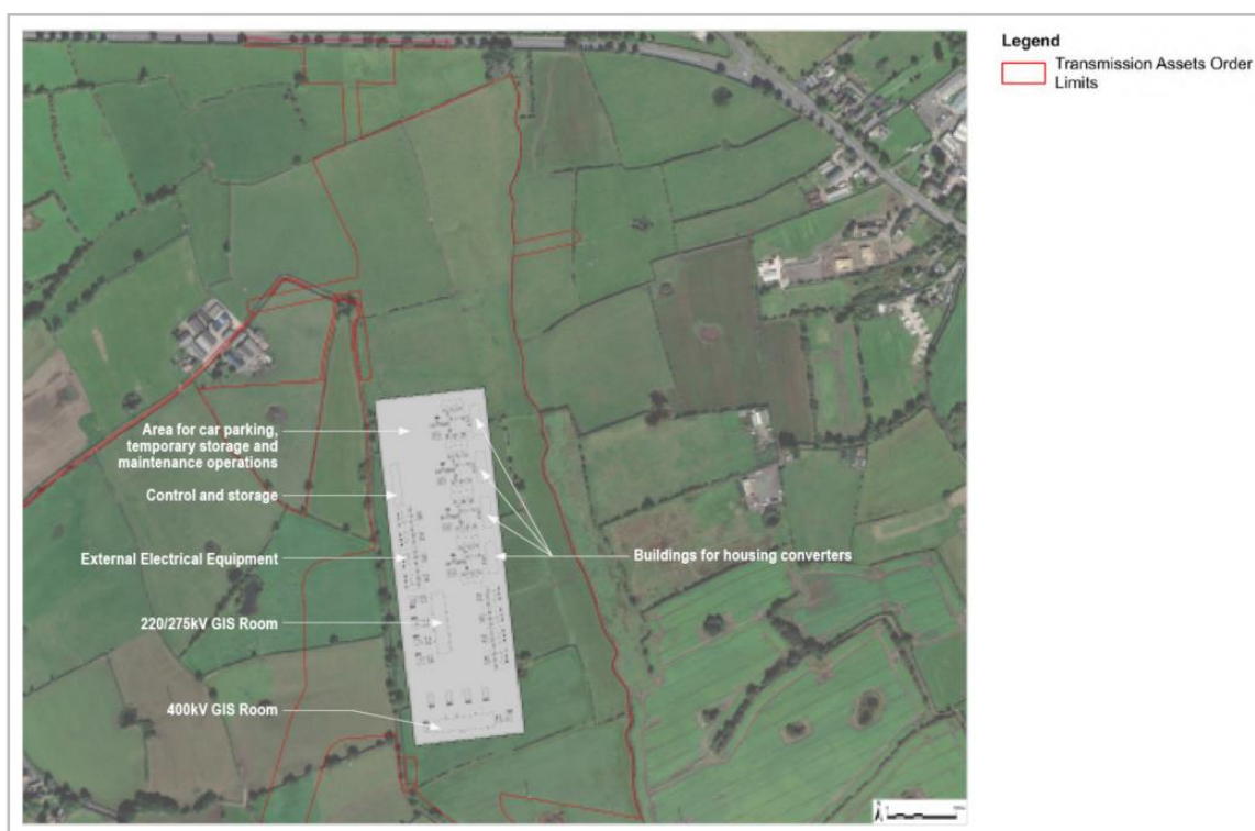
Figure 14: Indicative layout of the substation, Morecambe
