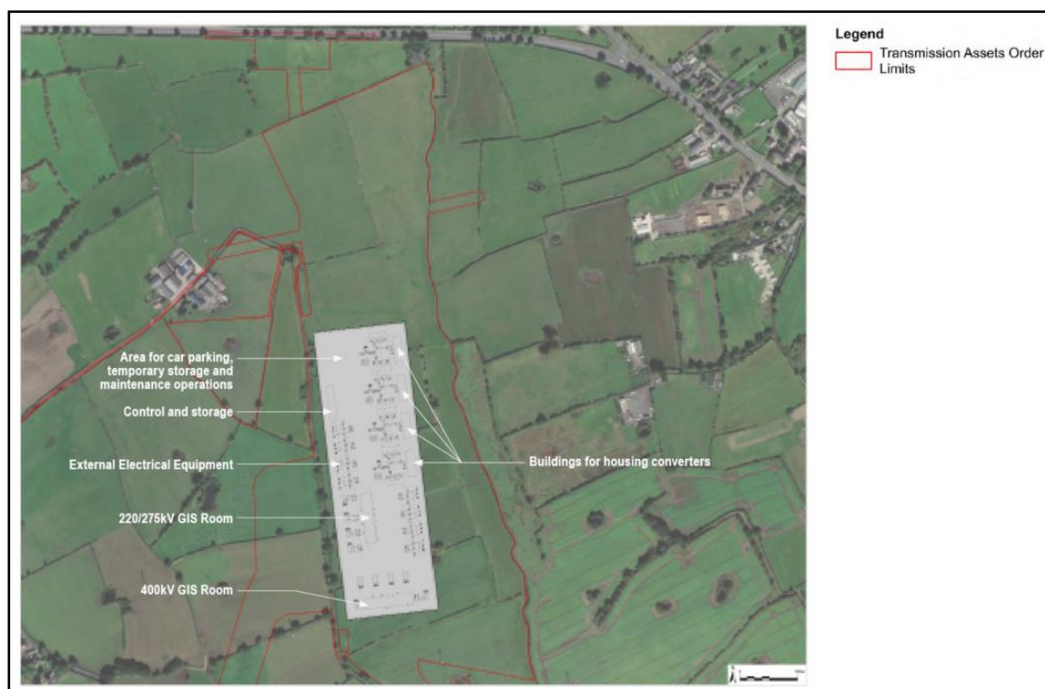
Figure 24: Indicative layout of the substation, Morgan
