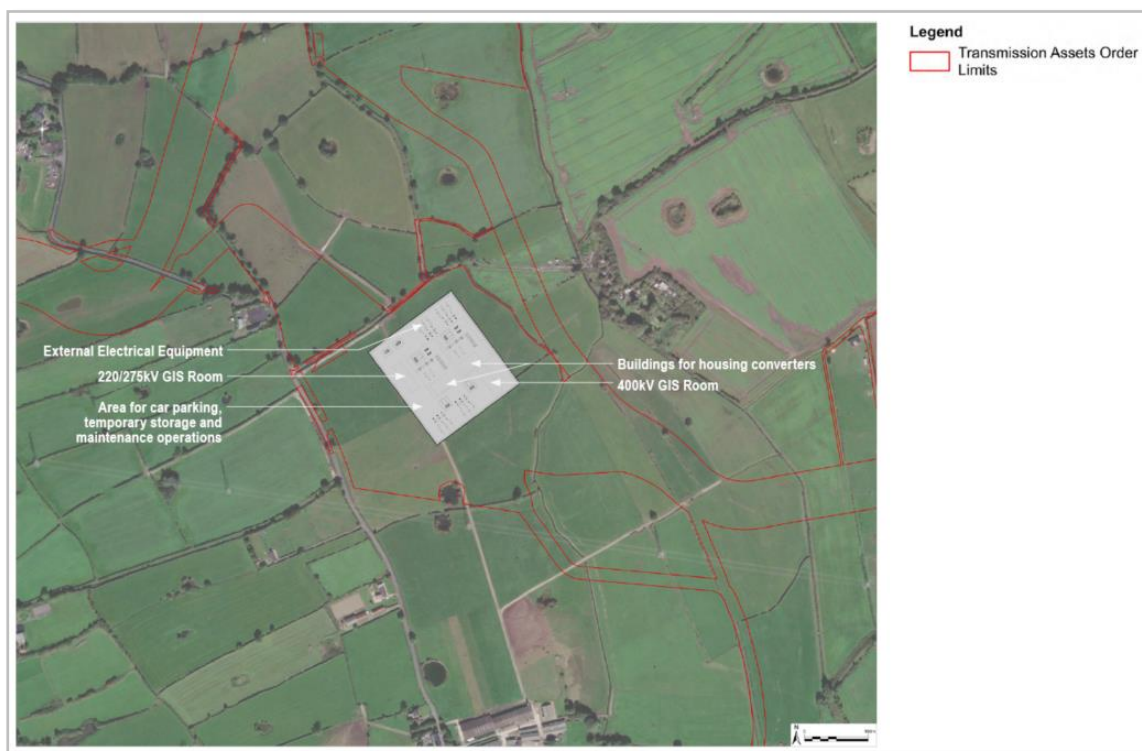
Figure 14: Indicative layout of the substation, Morecambe
